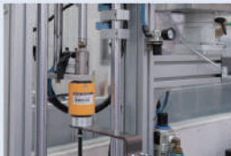
氣壓棒效能測試 (壽命 & 應力) Gas spring performance test (useful time & stress test)
