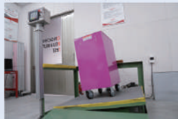
腳輪煞車力測試 & 產品穩定度測試 Casters brake test & product stability test
